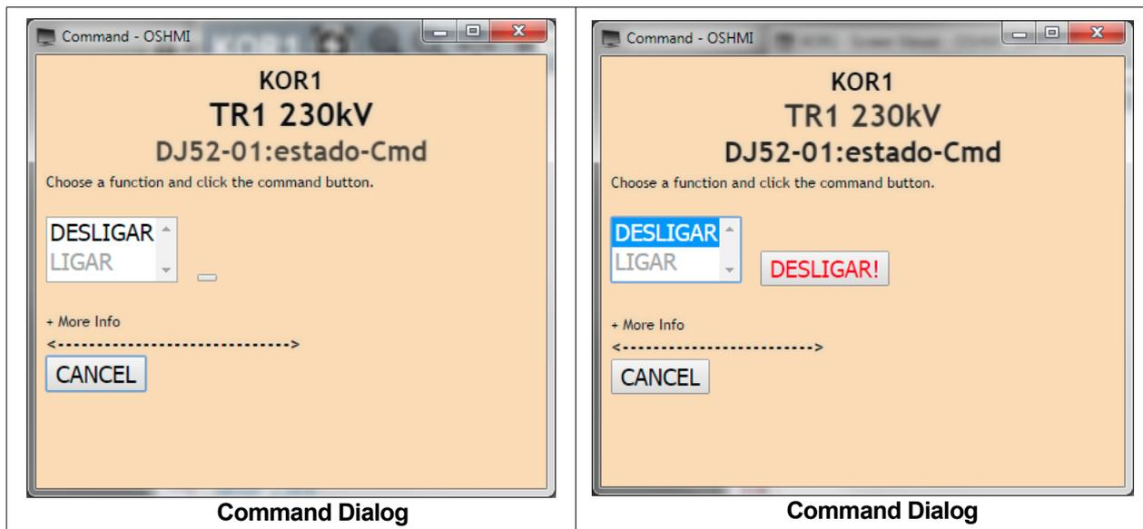
To reach the command dialog, first open the Point Info Dialog by clicking the desired object to be commanded, then click the "COMMAND" button.
